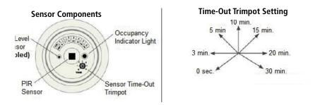
After confirming system is working normally, set controls to desired delay. Delay is the time that will elapse before fixture switches from white to Indigo-Clean mode.
