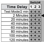
5. **PIR Sensor:** (for confirming operation you may want to set [Time Delay] to position "1" to shorten delay.)
