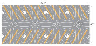
8 Fixtures @ 30' Spacing 10' Ceilings Fixtures mounted 8'.3" from floor
