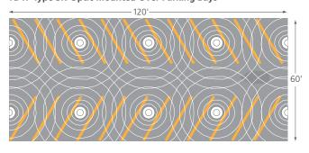
8 Fixtures @ 30' Spacing 10' Ceilings Fixtures mounted 8'.3" from floor
