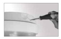
1. Remove three (3) screws on housing to open.
